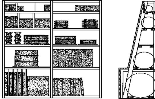
As illustrated above proper storage of grinding wheels prevents damage due to handling errors. Treat all grinding wheels with caution and use plastic or paper blotters. A cracked grinding wheel can explode and cause serious injury or fatality. Prior to storage, vitrified bond wheels should be spun dry after shutdown of coolant. If the wheel is removed from the wheel flange inspect the area of the wheel bore prior to the next use.
