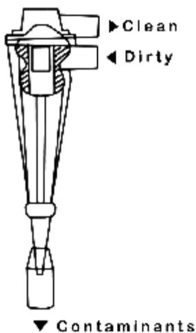
Hydro-cyclones are similar in operation to a centrifuge and operate on the following principal. Dirty coolant is carried through the slurry inlet. Rapid rotation of the dirty coolant overflows to the clean outlet while solids are rapidly moved by the vortex inside the cone. Then the solids are forced through the exit orifice at a reduced flow.
