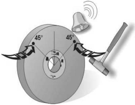
When using a conventional vitrified grinding wheel, it is necessary to check for cracks prior to mounting the grinding wheel to the flange. Cracks can occur due to improper storage and/or handling of the brittle structure of the wheel. The preferred method of testing for cracks is to perform a ring test, paying careful attention to the sound the wheel generates when struck.
