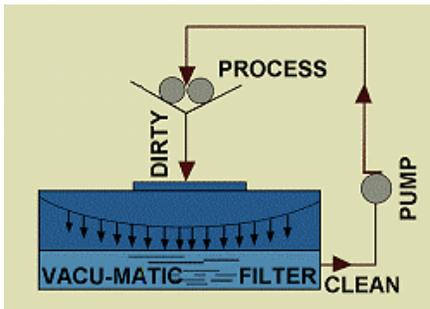
The vacuum system uses a suction pump to pull contaminated liquid to the filter paper located in the bottom of the tank. Once the cake of material has built up and liquid can no longer pass freely a vacuum level is detected, the suction pumps cycles off and the conveyer moves the swarf and filter paper up a ramp to dry before discharged.
