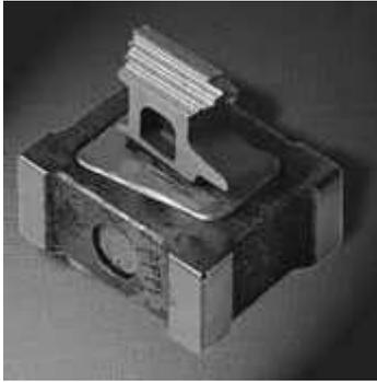
Encapsulating the aerospace turbine blade is one of the typical methods used for fixturing.
