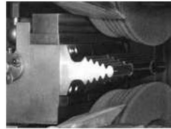
Another effective solution to coolant application is the use of coolant ramps on each side of the part machined to promote coolant penetration in the arc of cut. The formula below will assist in making this determination to coolant nozzle size.
