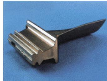
This illustration is of a blade that has been finish ground and removed from the encapsulated block. Typically a break out die is used to separate the blade from the zinc. The zinc can then be recycled for later use.
